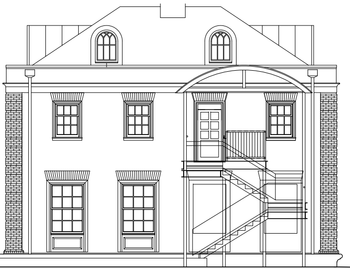
2 NEW STAIR - EAST ELEVATION SCALE: 1/4" = 1'-0"
